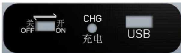
Use Type-c interface to charge, The indicator light is on when charging, The indicator light goes out after full charge, Toggle switch ON/OFF the device
